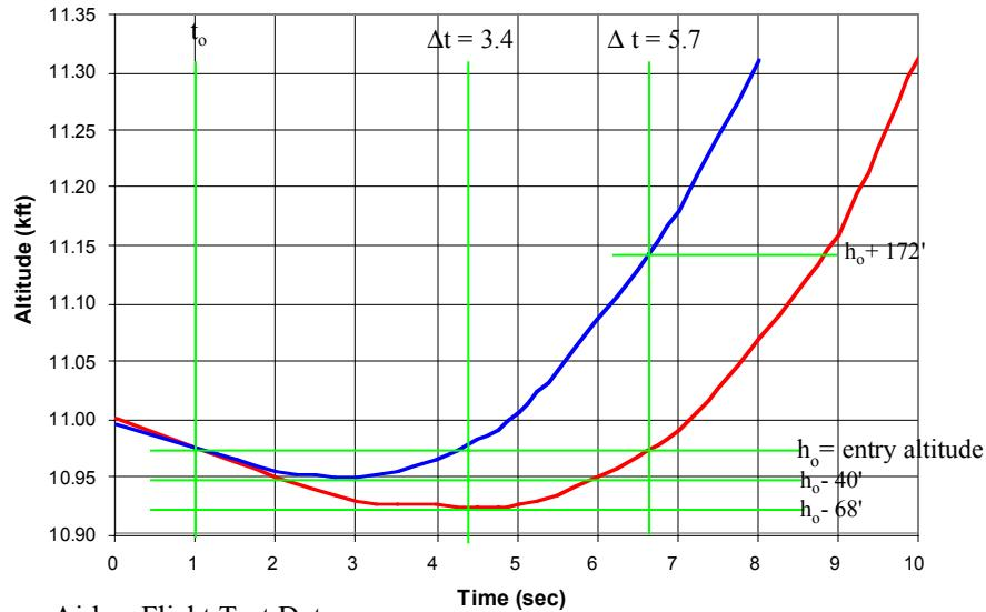
Source: Airbus Flight Test Data
