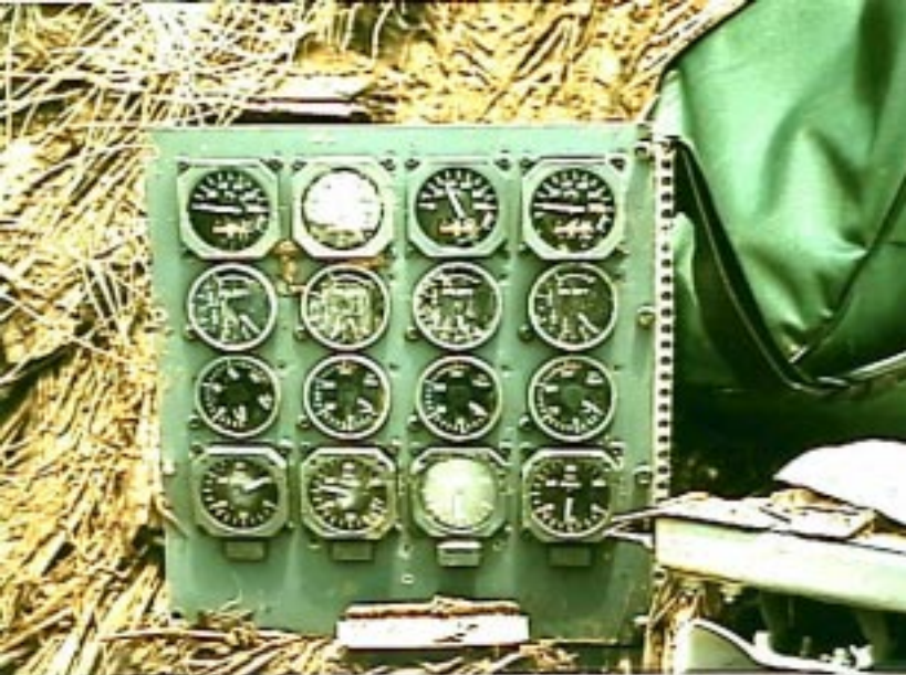
Photo 19: Flight Engineer's Engine Instrument Panel
