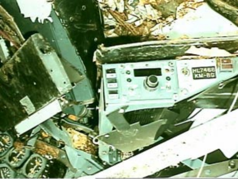
Photo 14: Right Side VHF Control Panel
