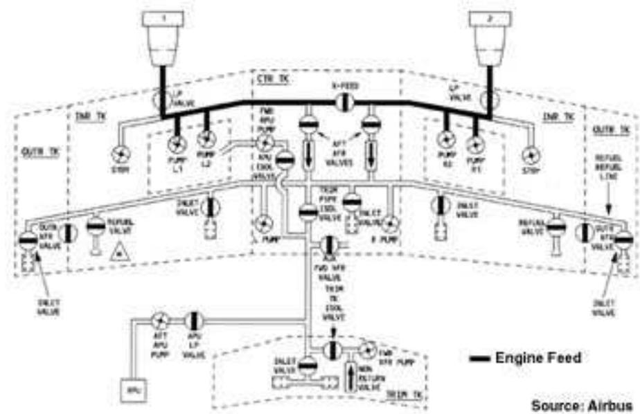
Figure 1: Fuel Schematic for the A330 (from [])
